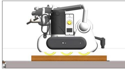
5. Connect the feeder to the power supply and confirm correct feeding.
